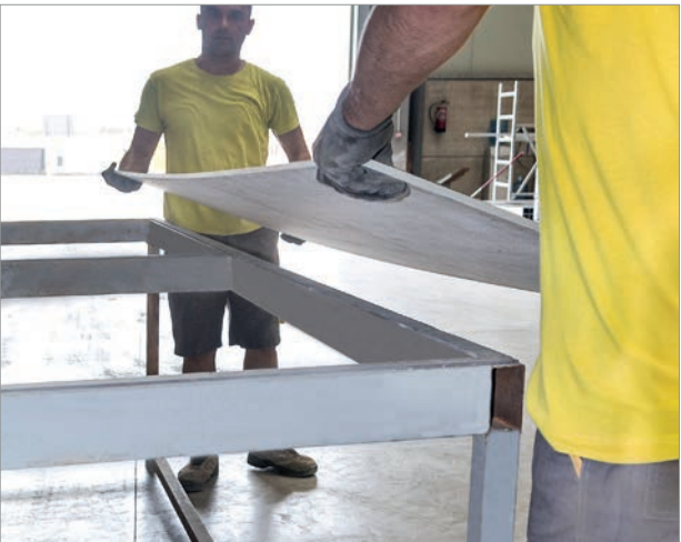
Image 8: Placing a Neolith Slab on a bench
