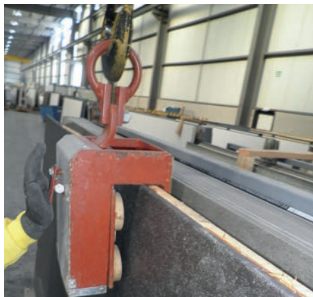
Image 4: Handling with Clamp
