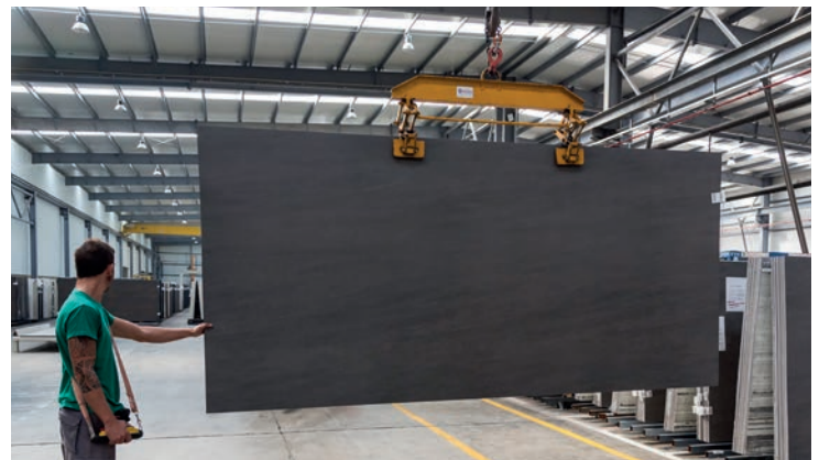
Image 2: Neolith slab handling with Clamp
