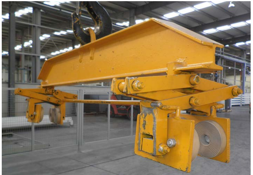
Image 9: Clamp handling for 12 mm slabs
