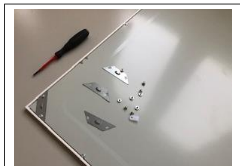
Fig 31 Commercial LED panel: removal of fixtures on the back of the panel
