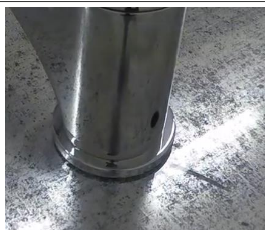
Fig 5 Example of excessive tightening
