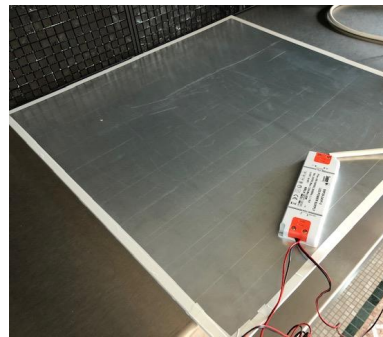
Fig 29 Example of customized LED panel - backside
