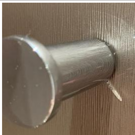
Fig 11 Example of excessive tightening
