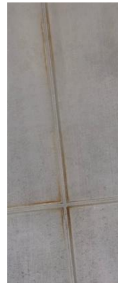
Fig 37 Example of contamination from tin
