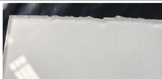
Fig 15 Example of edge resulting from a Waterjet cut in which too little abrasive was used and cut speed was too high – lower glass layer
