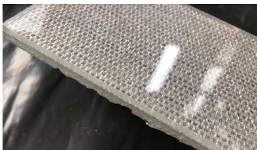
Fig 14 Example of edge resulting from a Waterjet cut in which too little abrasive was used and cut speed was too high – upper glass layer
