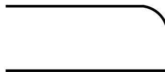
HALF-BULLNOSE EDGE 12/20 MM CANTO SEMI-REDONDO 12/20MM
